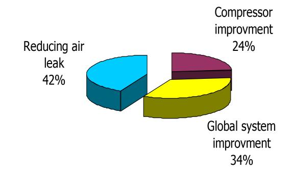
The largest contributor to energy efficiency is to reduce air leaks
