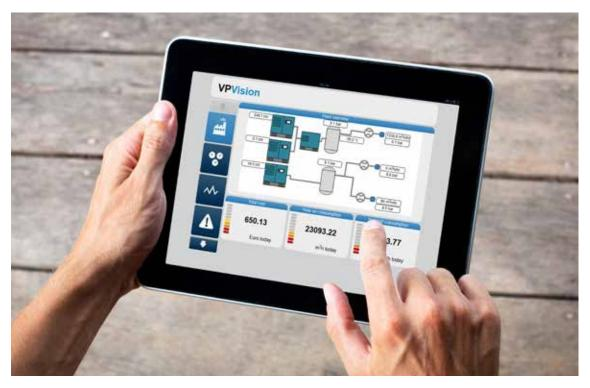
In the P&ID module you can place real time widgets on a background diagram.
